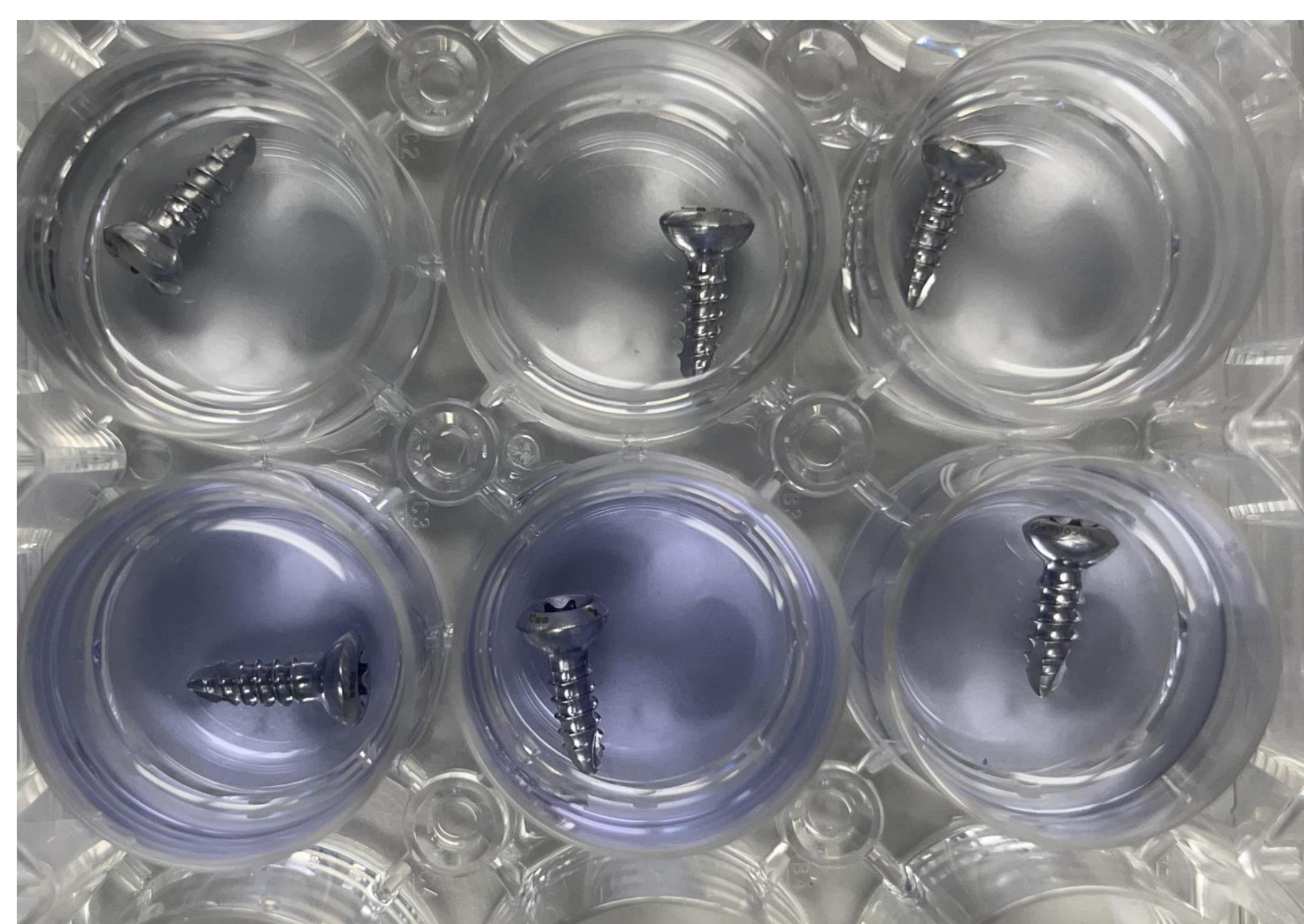
Bromelain powder + scrub treatment group (top row) resulted in less crystal violet-stained residual biofilm versus Control Screws (bottom row)
