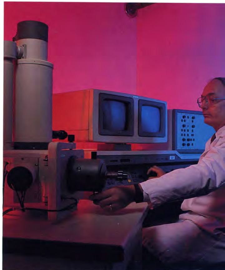
Dr. Roger Beuerman studies nerves of the eye's surface with the scanning electron microscope.
