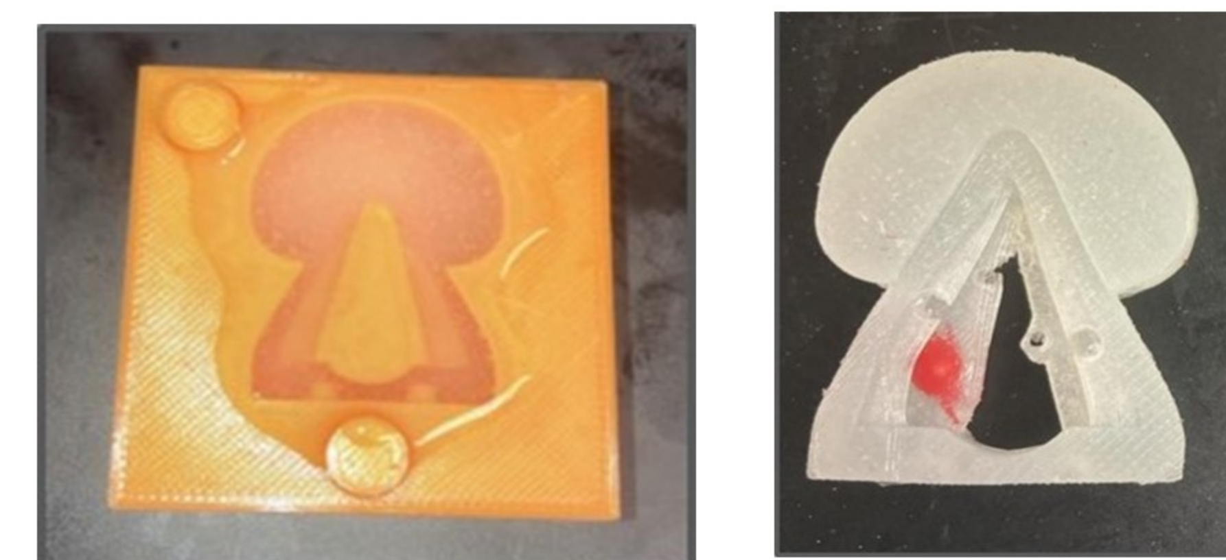
Figure 3: Synthetic larynx model. (A) Negative TPU mold; (B) EcoFlex silicone vocal fold with tumor phantom.
