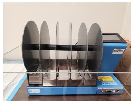
**Figure 4. Picture of rotarod apparatus for mice.** Mice are placed in individual lanes at a baseline rotation of 4 RPM that accelerates to 40 RPM over 240 seconds. Three trials per mouse separated by a 10-minute rest period were recorded and the average latency to fall was calculated. Mice had been previously acclimated to the rotarod using the same testing paradigm 2-3 days prior to the experimental run.
