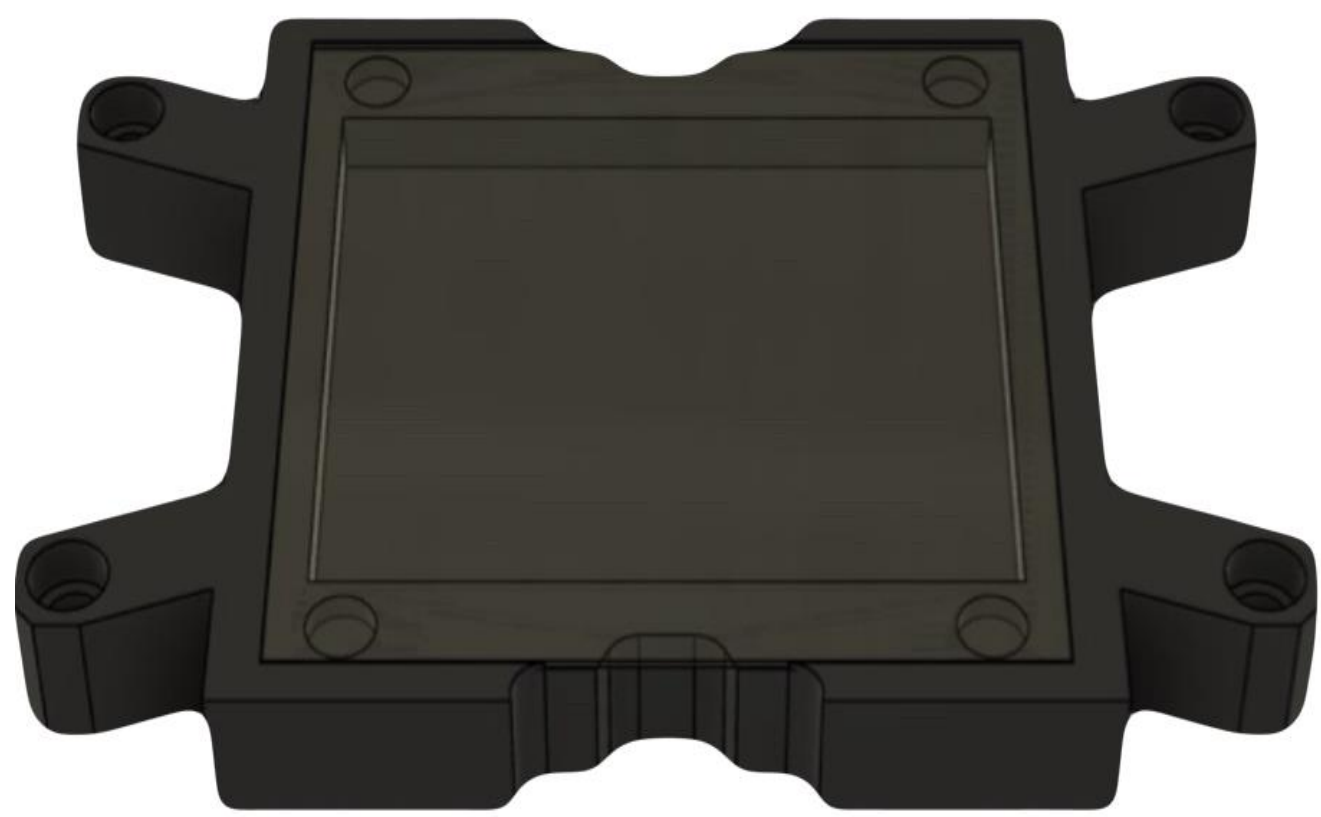
Pictured above is a Fusion360 model of a sample holder with a 10cm x 10 cm glass slide
