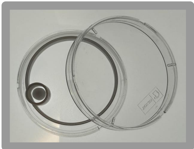
Figure 1: Calcium bead secured with PLA insert in 35mm plate.
